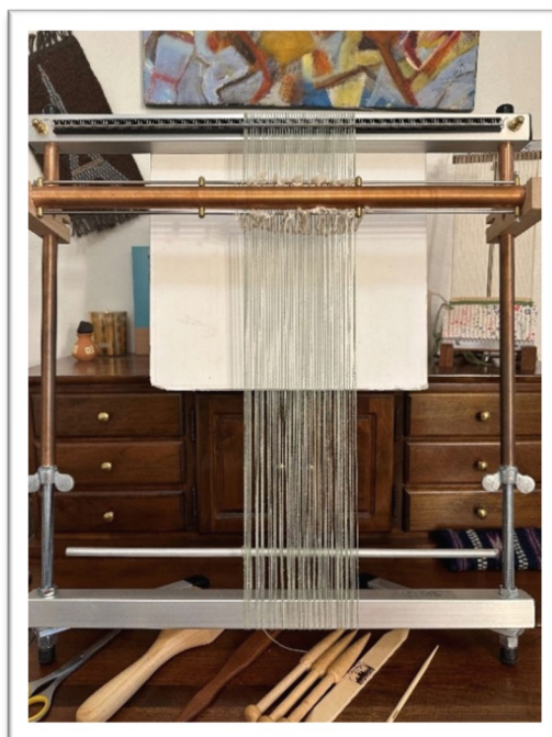
22" Mirrix Zach Loom, which has a shedding mechanism
