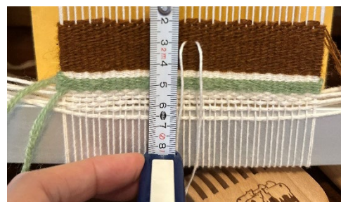
First 20 picks slightly compacted after weaving an additional 10 picks ( \approx 1.3\text{--}1.5\text{ cm} / 0.51\text{--}0.59\text{ in} ), beaten with a beater.
